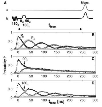
times, and microwave cross talk. (C) Plot of measurement probabilities for a sequence that creates the eigenstate  $|\psi_2\rangle=(|01\rangle-|10\rangle)/\sqrt{2}$  of the coupling Hamiltonian. After the eigenstate is formed by the  $90_z$  pulse, it ceases to evolve with time. (D) As in (C), but with an  $180_z$  pulse. Here, the phase of the oscillation changes by 180 degrees.
