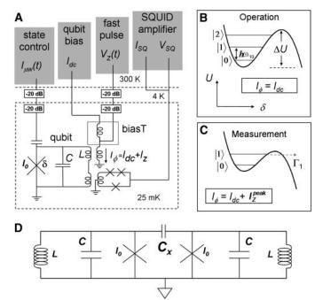
pulse, the energy barrier  $\Delta U$  is lowered to increase the tunneling rate,  $\Gamma$ , and the tunneling probability of  $|1\rangle$ . (D) Circuit diagram of the coupled qubits. The loop inductance, L, is  $\sim$ 850 pH, and the junction capacitance, C, is  $\sim$ 1.3 pF. An interdigitated capacitor with  $C_{\chi} \sim$  3 fF couples the qubits, giving rise to an interaction strength of magnitude S/h = 10 MHz.
