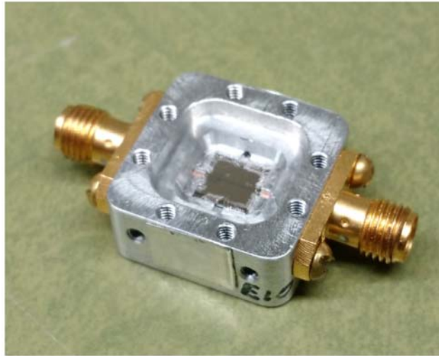
Figure 4.4: JPM wirebonded in aluminum sample box.
