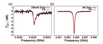
Figure 3. (Color Online) (a) Microwave transmission across an electroplated resonator measured at 100 mK. At single-photon power levels (shown), we find  $Q_{100~\rm mK}=1.5\times10^5$ . (b) Microwave transmission across a second electroplated resonator at 4.2 K. Note the different frequency scale. At this temperature, the internal quality factor is power-independent, with  $Q_{4\,\rm K}=3.0\times10^4$ .
