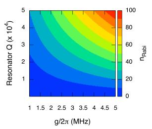
Figure 4. (Color Online) Surface plot of  $n_{\rm Rabi}$ . For the demonstrated resonator quality factor of  $3.0 \times 10^4$  and a coupling  $g/2\pi = 3$  MHz, we expect to achieve  $n_{\rm Rabi} \approx 35$ .
